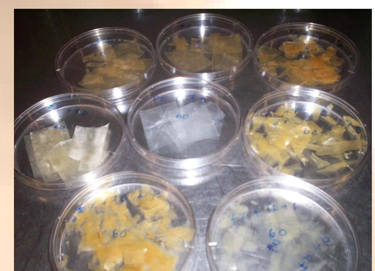
Figure 8. Photo-degraded samples of PE and its nanocomposites
