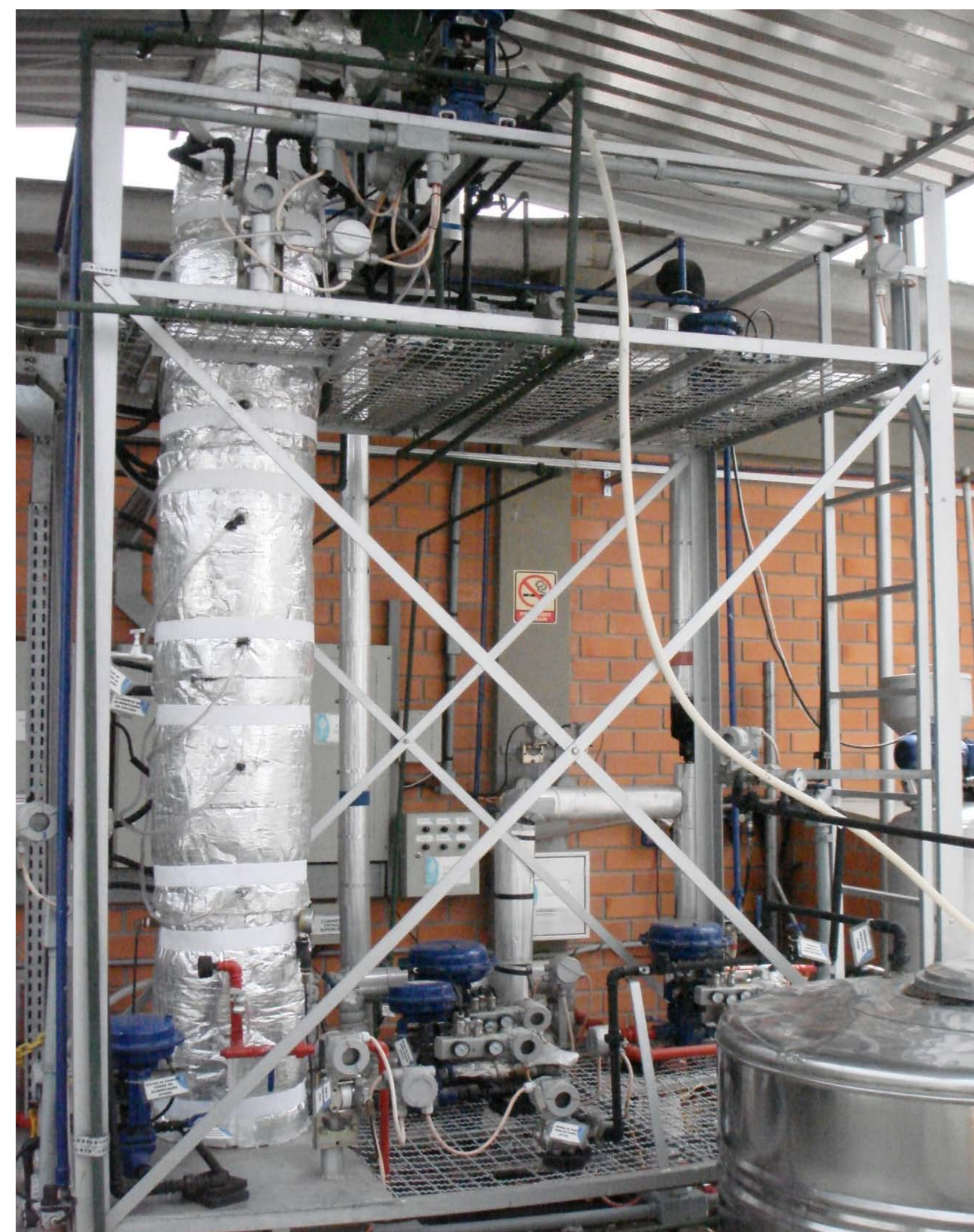
Figure 1 - Pilot distillation unit.
